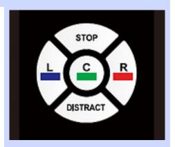
The "STOP" button on the remote supresses activation from the button in the event the patient presses when not desired.
