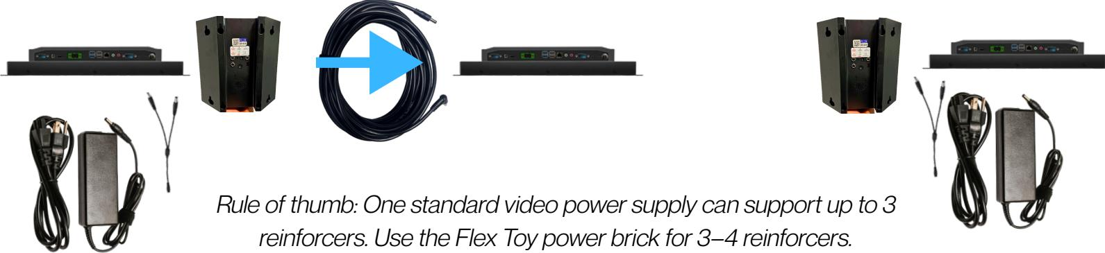
*Rule of thumb: One standard video power supply can support up to 3 reinforcers. Use the Flex Toy power brick for 3–4 reinforcers.*
